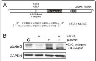
**Figure 1** The replacement strategy tested for *ATXN3*. (A) The target site and nucleotide sequence of siRNA directed at the *ATXN3* transcript. (B) The western blot analysis of the ataxin-3 levels in the HeLa cells at 72 h after transfection with 100 nM siRNA SCA3 and/ or ATXN3-8Q plasmid. C - the reference line shows the *ATXN3* expression level in the cells transfected with control siRNA. The GAPDH protein level was used as a loading control.
